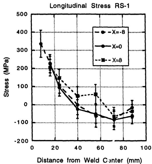
Figure 2. A plot of the longitudinal residual stresses in the RS-1 plate (as-welded) at the top (X=-8), middle (X=0), and bottom (X=8) of the plate. The distances are measure from the center of the fusion zone in the plate.
